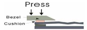
13.3 The area from Viewing Area 2mm is structurally weak for pressure, especially for pen use, the film may be forcibly bent and cause defection. This area must be protected by the bezel and input must be avoided.
